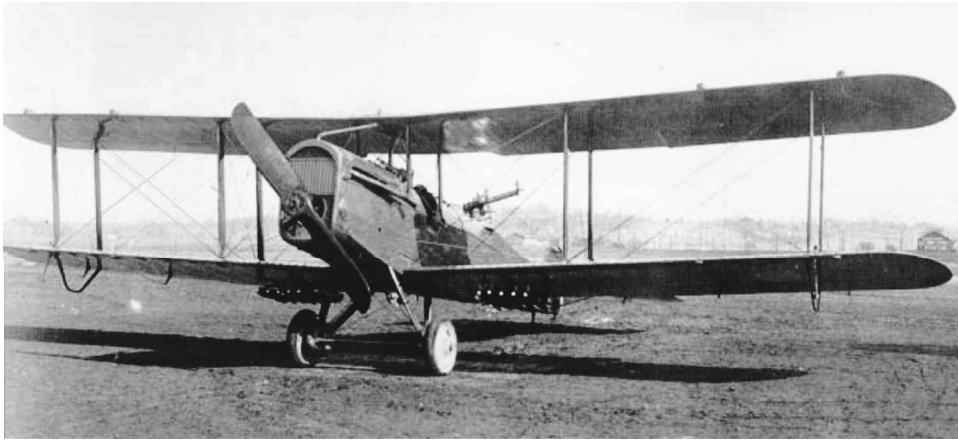
Fig. 3 American-built de Havilland DH-4 with wood propeller and 400 hp Liberty engine.
