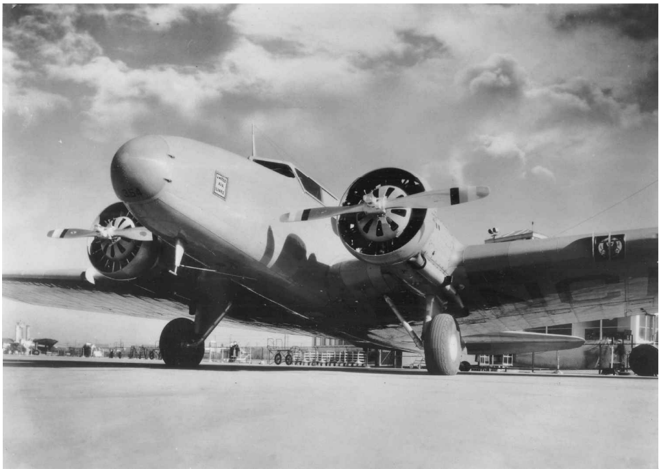
Fig. 10 Modified Boeing Model 247 with two-blade, two-position, controllable-pitch propellers.
