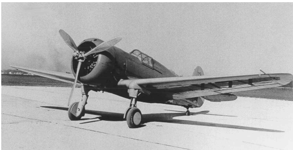
Fig. 12 Curtiss Y1P-36 with Hamilton Standard constant-speed counterweight propeller, 1937.
