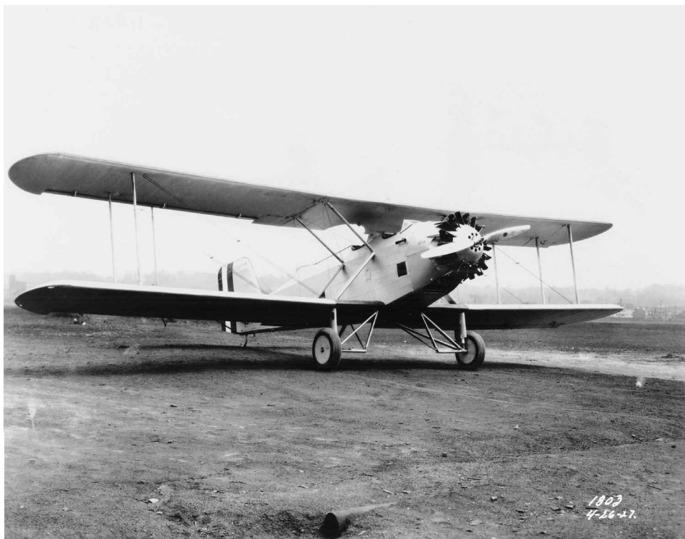
Fig. 5 Martin T4M-1 torpedo-bomber scout with Standard Steel dural ground-adjustable pitch propeller.
